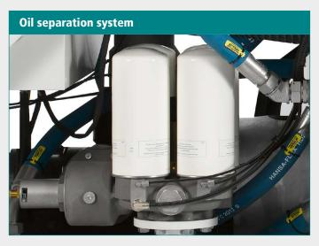
Compressors up to 127 kW are equipped with three or four external separator cartridges which can be changed by a simple spin-off/spin-on procedure. Thanks to the outstanding separation efficiency of the entire system, the compressors can be used in the pressure range from 5,0 to 15,0 bar.
