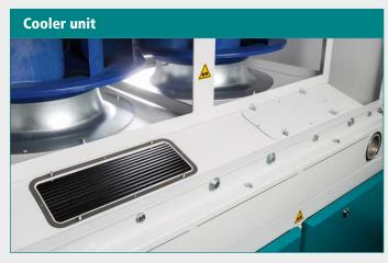
The horizontally mounted cooler can be cleaned by cleaning lids. Alternatively the cooler can be pulled out like a drawer for the purpose of cleaning. Thanks to well dimensioned after coolers for oil and compressed air as well as the integrated oil temperature control, the compressors run reliably even at high ambient temperatures.
