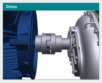
1:1 direct drive connects the air end directly to the motor. The almost loss-free power transmission guarantees reliable, high-performance compressor operation. The regular maintenance requirement is reduced to lubrication of the motor. All the electronic components are branded products of leading manufacturers.
