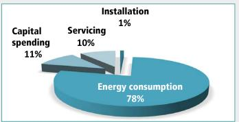
After 5 years of operation, the energy cost usually amounts to 78% of the total cost of a conventional compressor. The only way to reduce the overall cost is to reduce the cost of energy.
